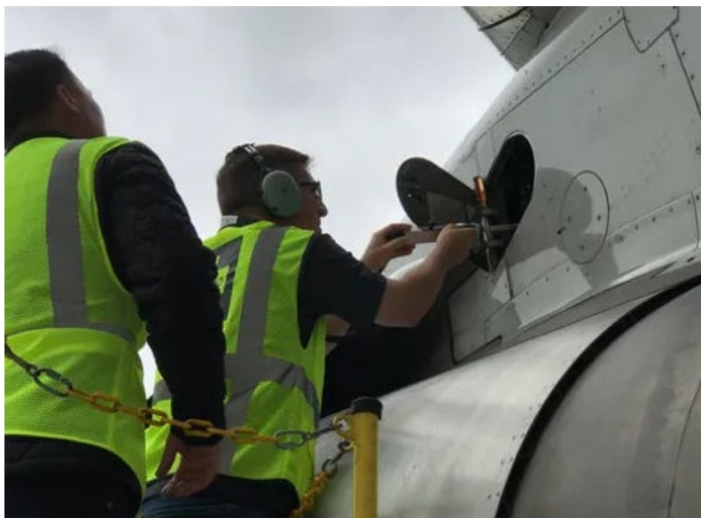
A member of Boeing's maintenance and ground operations systems uses the UL101 Troubleshooter to perform a bleed air check on a Boeing 757 © CTRL Systems
